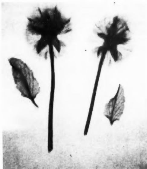
Fig. II-14 Radiograph of pansies and leaves made with an Fe^{55} source in a helium atmosphere. Time, 4.5 hr. Film, Polaroid 3000 X.
